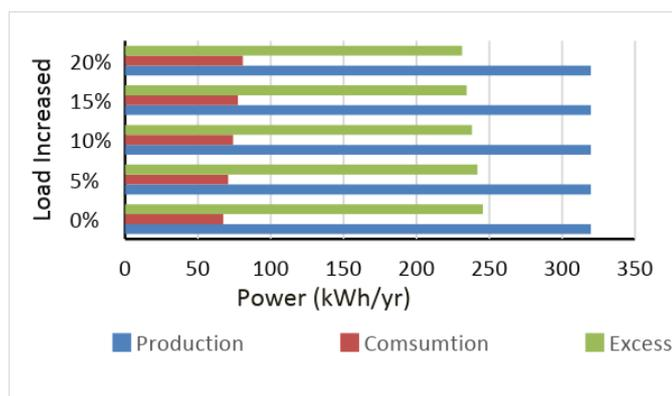
Fig. 6 Comparison of total electricity production, total electricity consumption, and excess electrical energy generated from load growth.
