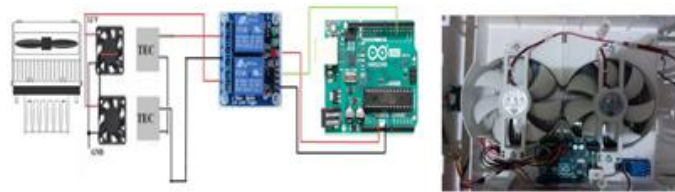
Gambar 4. Peltier TEC12706 ke Arduino
