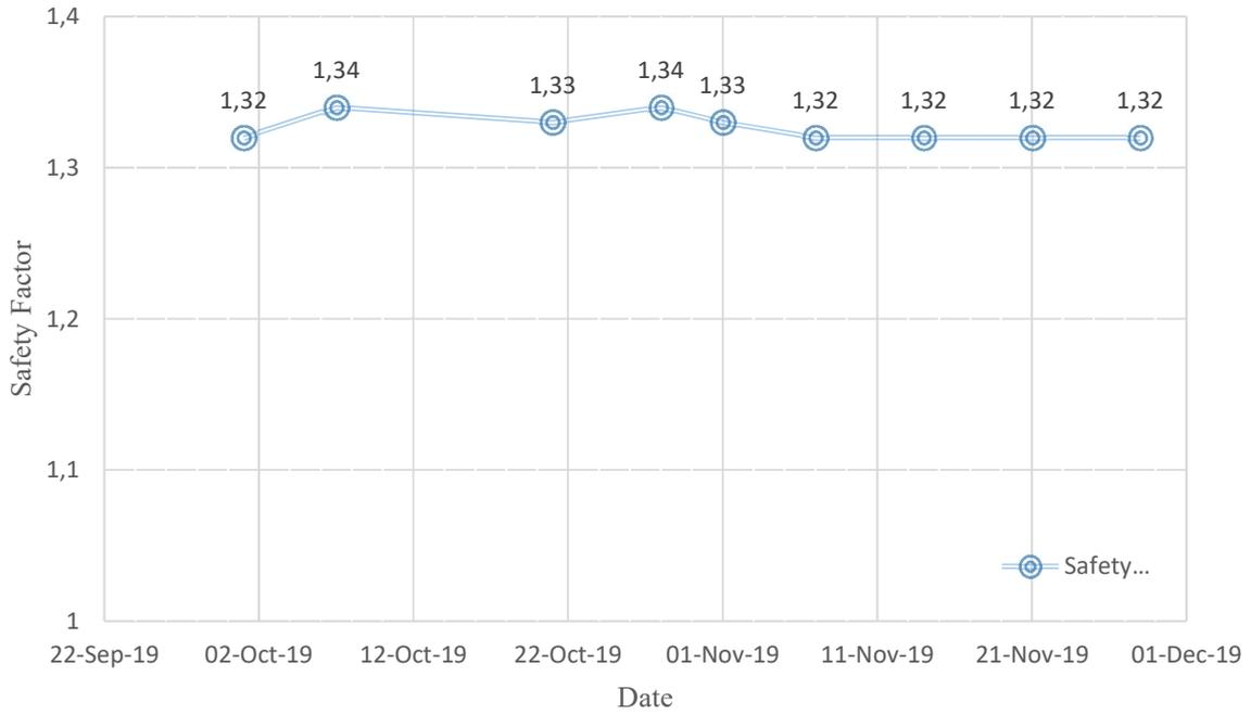
FIGURE 6. Result of the slope stability analysis (weekly) for two months.
