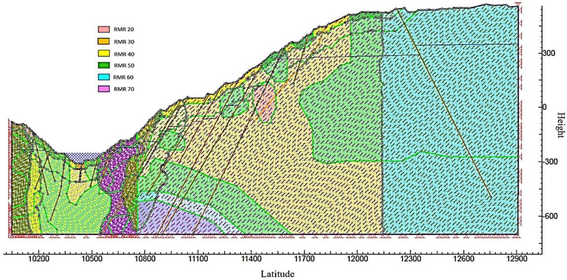
FIGURE 4. Anisotropic rock mass model of the North-East (section 20) for slope stability analysis with rock mass rating, discontinuity, and fault data.
