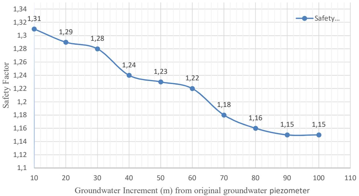
FIGURE 7. Result of the slope stability analysis after the increment of the groundwater table.
