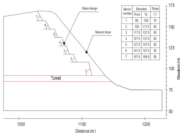
FIGURE 2. Natural and designed tunnel portal slopes.
