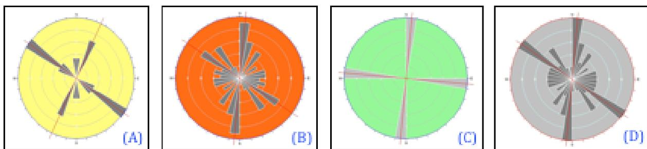
Figure 2: Principle Discontinuity orientation: (A) Sandstone, (B) Granite, (C) Mudstone, (D) All unit of rock.
