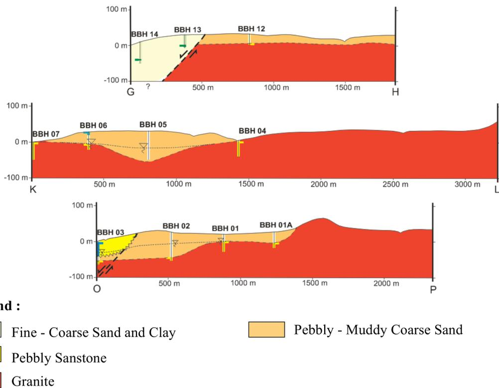
Figure 4: Engineering geology map cross-section G-H, K-L and O-P.
