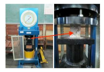
Figure 6: Uniaxial Compressive Strength (UCS) equipment.
