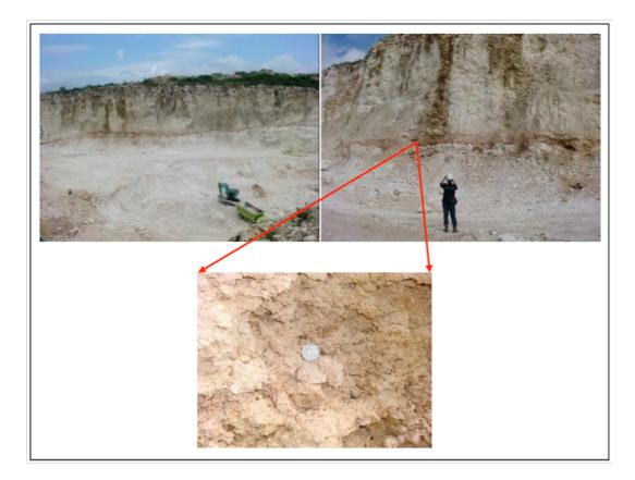
Figure 3: Cavity layer condition in limestone quarry.
