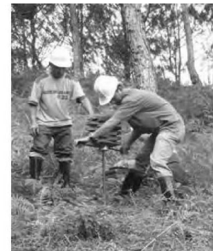
Figure 3: Swedish weight sounding test (SWST).
