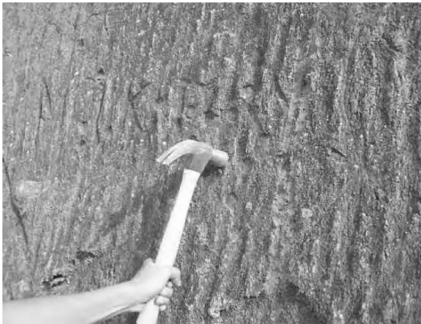
Figure 2: Hammer and nail test for estimating material classification in rock slopes.
