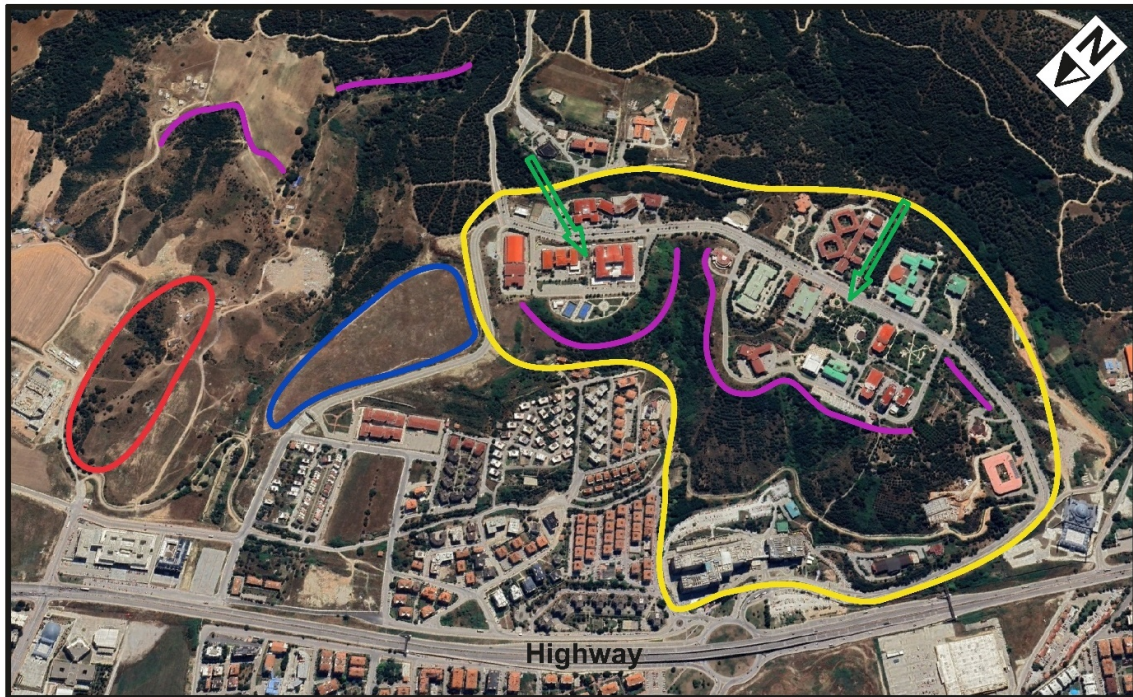
FIGURE 5. The study area (closed yellow line) and its vicinity are shown on a Google Earth image. The closed red line to the left indicates the area studied by Coşkun et al. (2016b). Çanakkale Municipality once used the location stated by the closed blue line for solid waste disposal. Purple lines show these likely landslide scarps. The highway links the cities of Çanakkale and İzmir.
