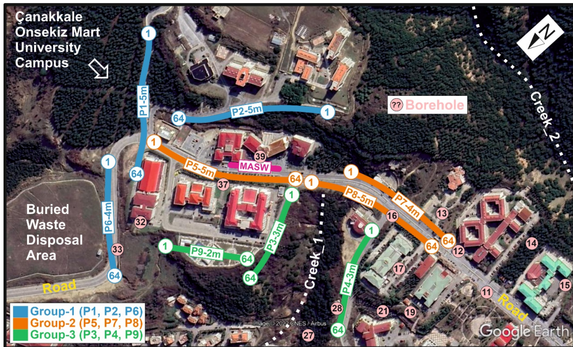
FIGURE 6. The ÇOMU campus and the electrical resistivity profiles indicated by orange lines are shown on a Google Earth image. Superimposed on the profile is the profile number and electrode spacing. The first (1) and last (64) electrodes are also specified. The seismic profile, which is a magenta color, indicates MASW. The two-digit borehole numbers are printed within circles with a pink color background.
