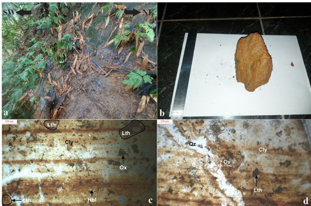
FIGURE 9. (a) Outcrop of lithic tuff. (b) hand specimen sample of lithic tuff. (c) Microphotograph of lithic tuff showing laminated structure. (d) Microphotographs of lithic tuff show a quartz vein filling the microfracture. Hbl = hornblende, Cly = clay, Ox = oxide minerals, Lth = lithic, and Qz = quartz.
