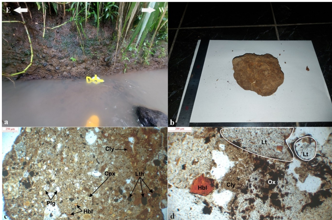
FIGURE 10. (a) Outcrop of tuff breccia. (b) hand specimen sample of the fragment of tuff breccia. (c) and (d) Microphotographs of tuff breccia. Hbl = hornblende, Plg = plagioclase, Cly = Clay, Ox = oxide minerals, and Lth = Lithic.
