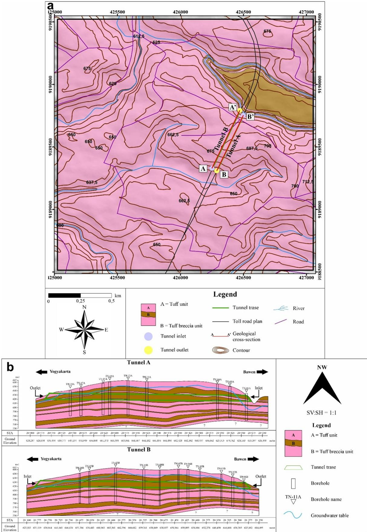
FIGURE 7. (a) Geological map of the study area. (b) Geological cross-section of the tunnel route.
