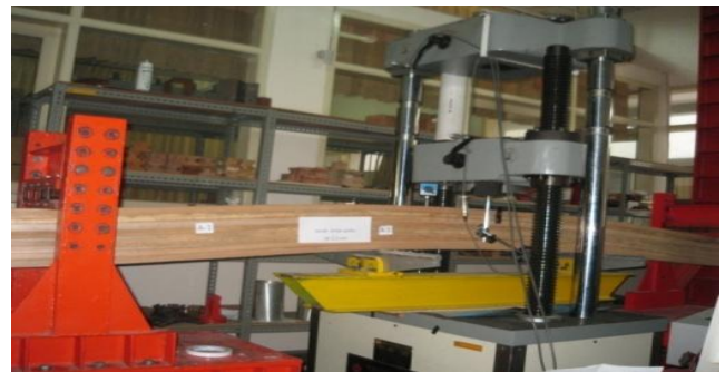
Figure 5. Third point bending test of a horizontally nail-laminated beam
