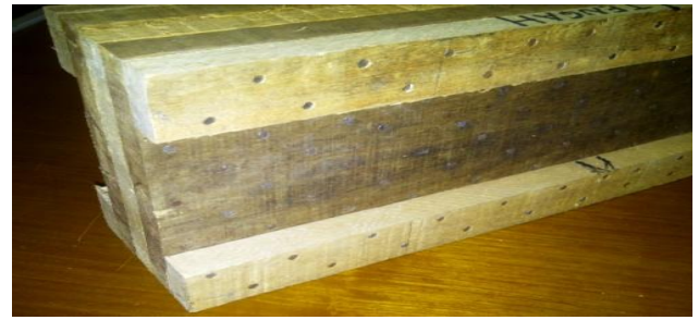
Figure 4. Nail spacing arrangement on vertically nail-laminated I beam
