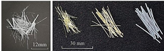
Figure 11. PVA, steel, aramid, and PP (from left)
