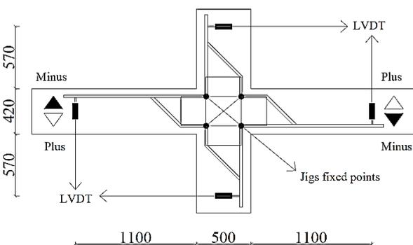
Figure 15. Measurement of beam and column local deformations
