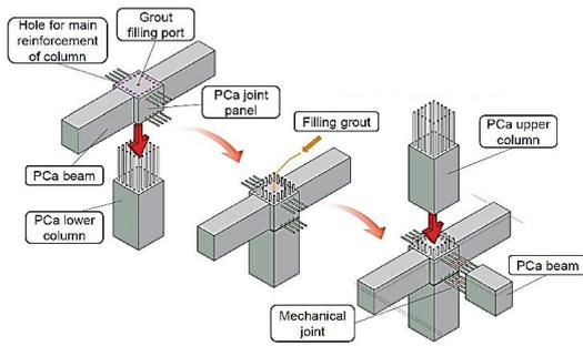
Figure 1. Precast system (Sano, et al., 2015)
