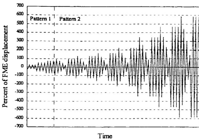
Figure 8. Sequential-phased displacement cyclic displacement (ASTM International, 2002)
