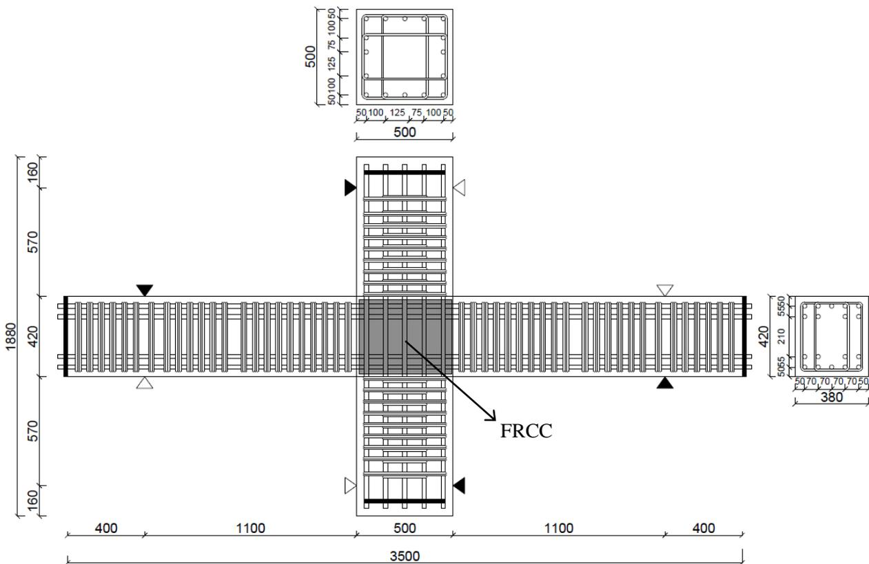
Figure 12. Specimen dimensions
