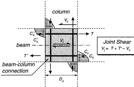
Figure 7. Horizontal joint shear in interior RC beam-column joint
