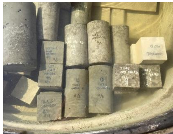
Figure 2. Curing of Concrete
