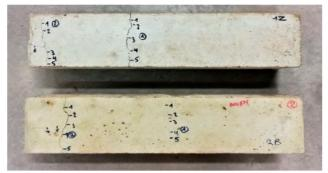
Figure 16. Laboratory prism specimens made by bioengineered concrete (Mullem *et al.*, 2020).
