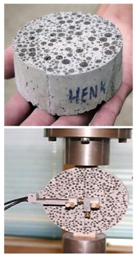
Figure 3. Bio-engineered concrete developed by the encapsulation method (Jonkers, 2011)
