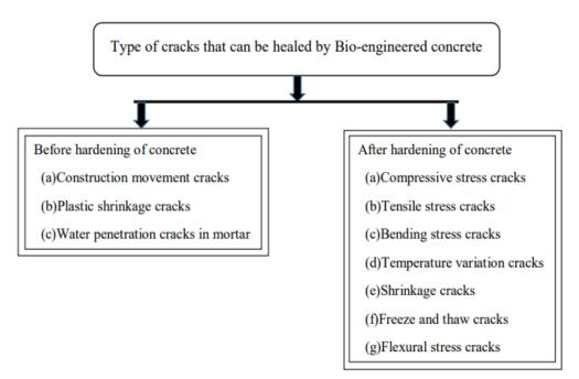
Figure 19. Type of crack healed by bio-engineered concrete.
