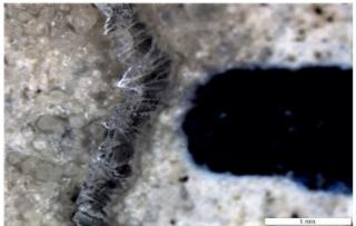
Figure 17. Formation of stalactites on a crack location of a prism specimen subjected to W/D cycles (Mullem *et al.*, 2020).
