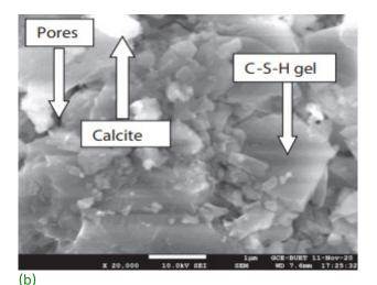
Figure 1. (a). SEM image showing the less dense microstructure of conventional concrete, (b). dense microstructure of bio-engineered concrete (Priyom *et al.*, 2020).
