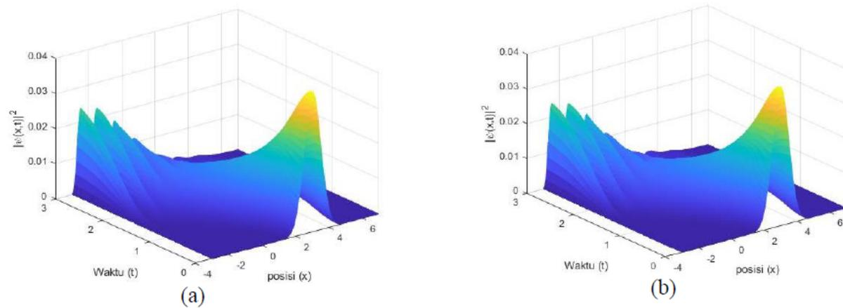
Figure 8: The solution  $|\psi(x,t)|^2$  using (a) Trotter – Suzuki decomposition second order and (b) second order hybrid with  $dx=0,05$  dan  $dt=0,001$
