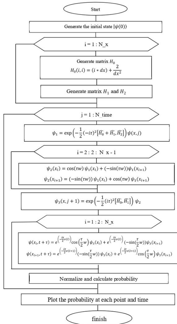
Figure 2: the flowchart of TDSE solution with Trotter – Suzuki hybrid second-order decomposition
