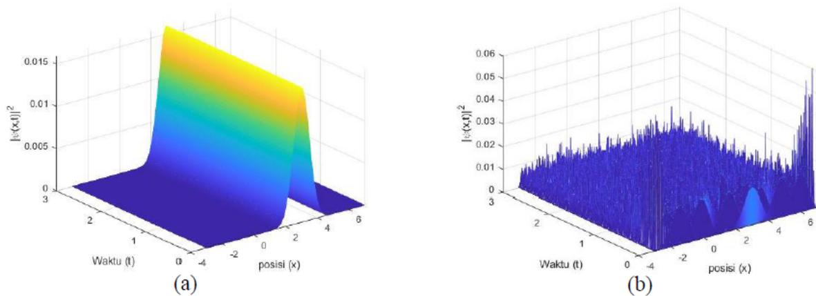
Figure 10: The solution  $|\psi(x, t)|^2$  using (a) Trotter – Suzuki decomposition second order and (b) second order hybrid with  $dx=0,02$  dan  $dt=0,01$
