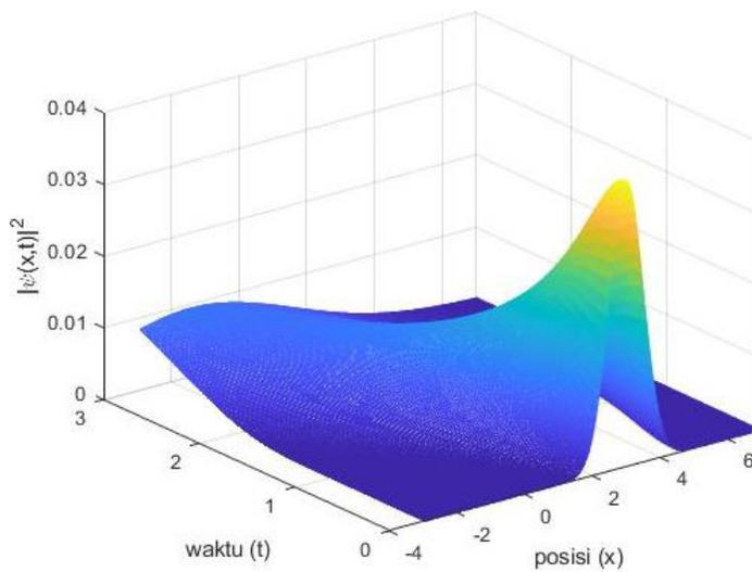
Figure 6: The solution  $|\psi(x, t)|^2$  using Baker – Campbell – Hausdorff method with  $dx=0,05$  dan  $dt=0,01$
