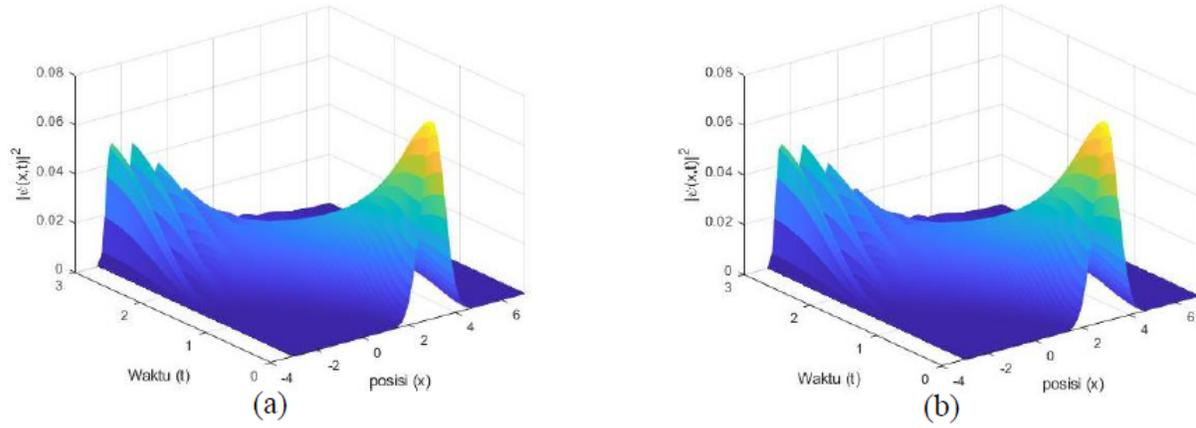
Figure 5: The solution  $|\psi(x, t)|^2$  using (a) Trotter – Suzuki decomposition second order and (b) second order hybrid with  $dx=0,1$  dan  $dt=0,001$
