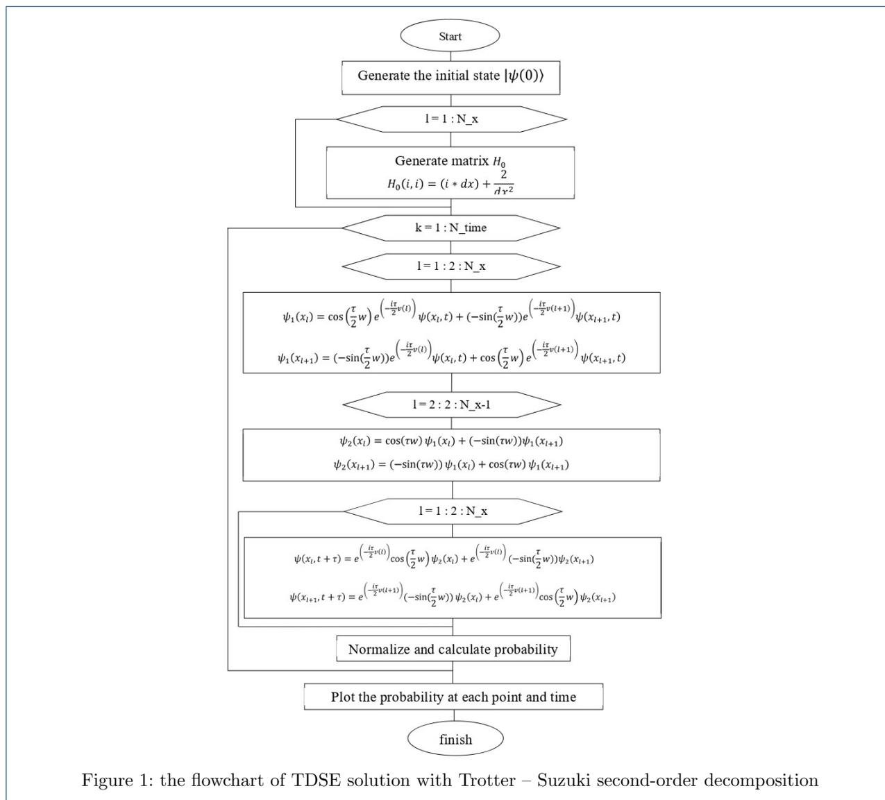
Figure 1: the flowchart of TDSE solution with Trotter – Suzuki second-order decomposition
