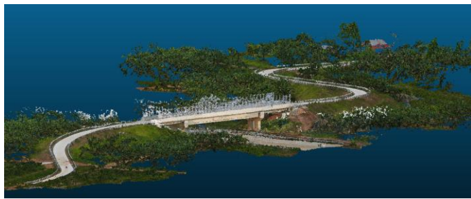
(a) point cloud sebelum filtering noise
