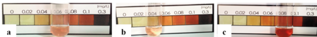
Figure 6. SST-kit application for cyanide detection of three cultivars of cassava : (a) Local; (b) CMM 6; (c) Adira 1 with triplicate experiments (n=3)
