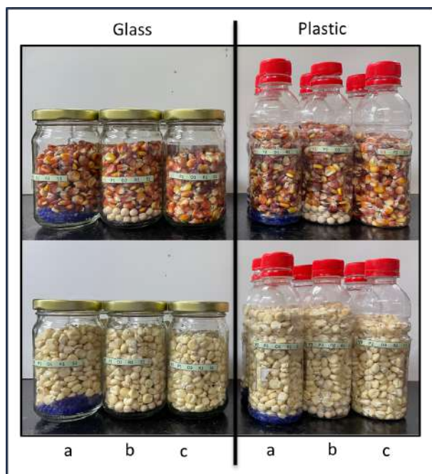
Figure 2. Storage set-up of organic corn seeds in glass (left) and plastic (right) bottles with silica gel (a), drying beads (b), and control or no desiccant (c).
