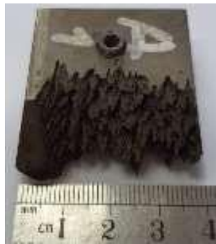
Figure 1. Erosion of the balance weight of the turbine
