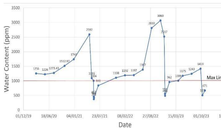
Figure. 5 Water Content (ppm) Trend in Ambient Humidity Without the Dehumidifier Box
