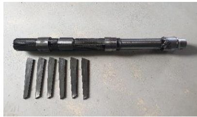
Figure 5. Adjustable Hand Reaming Tool
