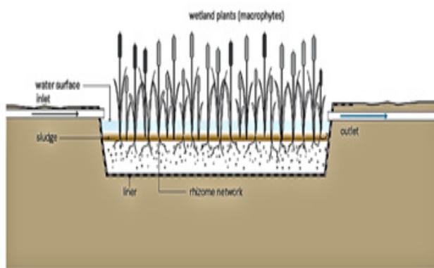
**Figure 2.** Profile of free water surface constructed wetlands
