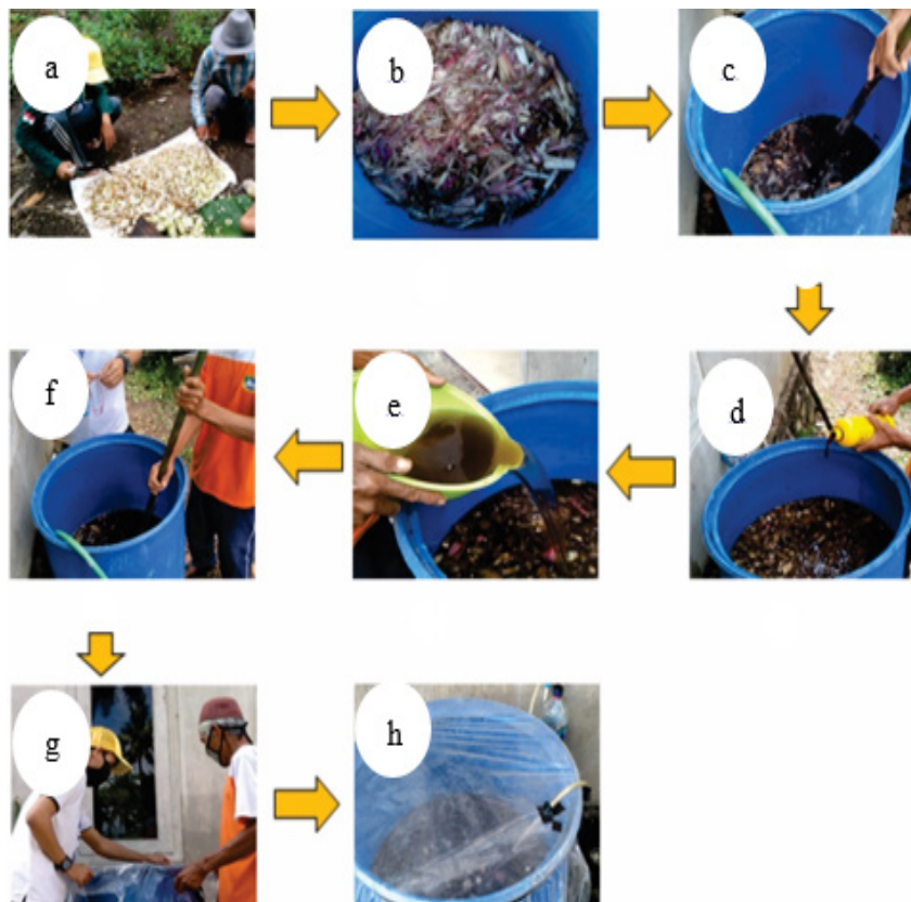
Figure 1. a) Chopping banana stem waste; b) Inserting chopped banana stem waste into a vat fermenter; c) Adding 50 litres of water; d) Adding 1 litre of EM4; e) Adding 1 kg of sugar solution; f) Stirring process to evenly distribute Material; g) Covers the fermenter with clear plastic and connects it to the aqua glass; h) The fermentation process is on progress
