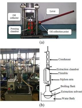
Figure 1. The process for obtaining oil from nyamplung fruit kernels, (a) by mechanical extraction, (b) by chemical extraction
