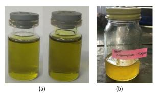
Figure 3. Nyamplung kernel oil, (a) before methanol extraction from mechanical extraction (left) and chemical/Soxhlet extraction (right), (b) after methanol extraction
