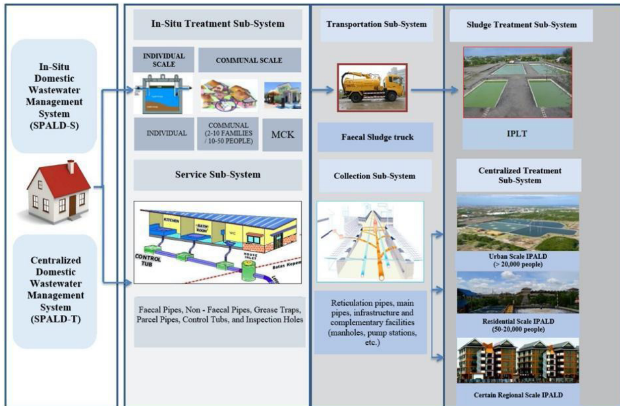
Figure 4. Domestic Wastewater Management Concept Based on Regulation of the Minister of Public Works and Public Housing No. 4 of 2017
