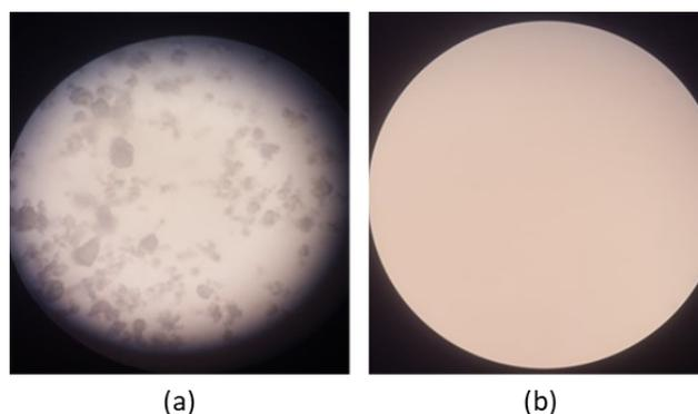
**Figure 5.** Microscopic images of precipitated calcium carbonates produced by *Bacillus cereus* viewed under light microscope (a)  $\times 40$  and (b) Uninoculated calcium carbonate precipitation medium.
