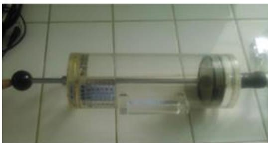
Gambar 7. Syringe berukuran 2000 ml
