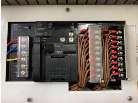
Gambar 2. PLC Omron CJ2M-CPU31
