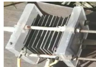
Gambar 4. Generator kering HHO (*dry cell*)
