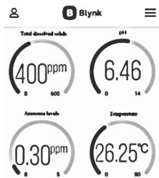
Figure 9. Results of water quality parameter measurement on the Blynk IoT interface application
