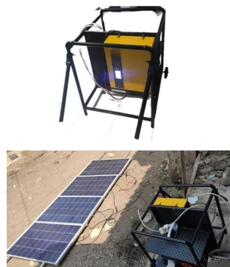
Figure 2. Portable power station with removable solar panels
