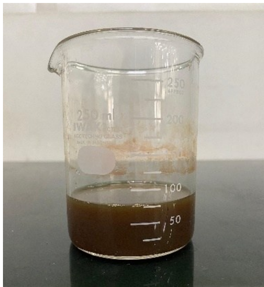
Figure 6. Appearance of silver nanoparticle solution after 30 days of storage in the refrigerator under dark conditions
