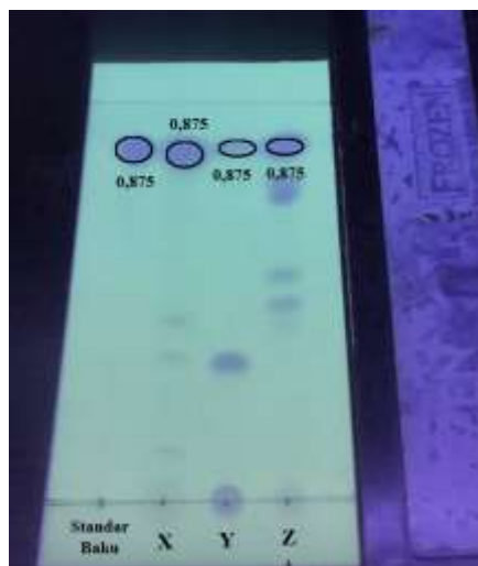
Figure 1. TLC Results of Facial Sunscreen Gel Samples Under 254 nm UV Light (Standard Solution; Sample X; Sample Y; Sample Z)
