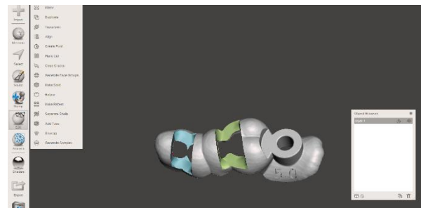
Figure 4. Design process for window on dental implant guide
