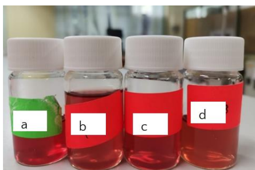
Fig. 11: Natural dye extracted at different extraction times where a) 30, b) 60, c) 90, and d) 120 minutes
