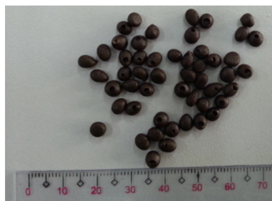
Fig. 1: Geopolymer spheres from coal fly ash and calcined waste pen shells
