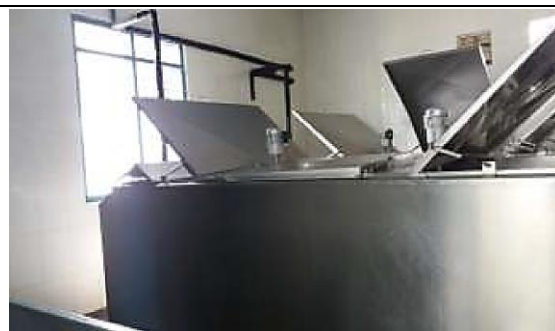
Fig. 1: Packo milk cooling tank (Courtesy of Koperasi SAE Pujon)
