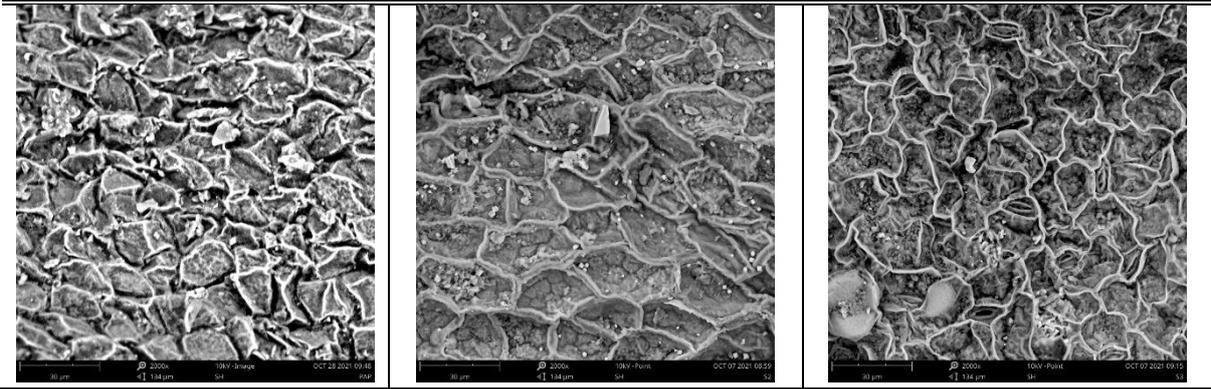
**Figure 5:** SEM scan of male papaya leaves (a) before the extraction process, (b) after the MAE process, and (c) after the UAE process under the scale of 30 µm and a magnification level of 2000x.
