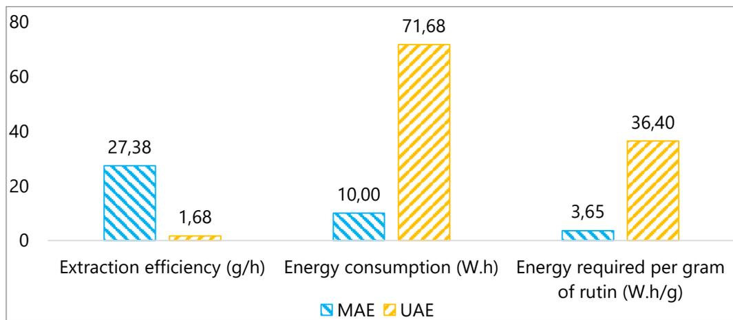
**Figure 6:** Extraction efficiency, energy consumption, and the energy required to produce 1 gram of rutin using MAE and UAE.
