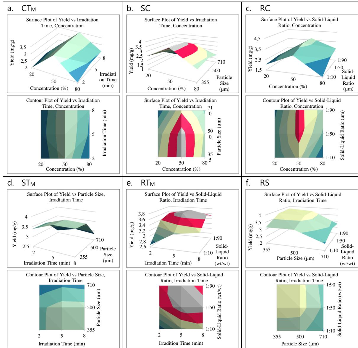
**Figure 3:** The surface and contour plots for rutin yield with MAE using male papaya leaves under the influence of (a) irradiation time and ethanol mixture concentration, (b) size of plant matrix and ethanol mixture concentration, (c) solid-liquid ratio and ethanol mixture concentration, (d) particle size and irradiation time, (e) solid-liquid ratio and irradiation time, and (f) solid-liquid ratio and size of plant matrix.
