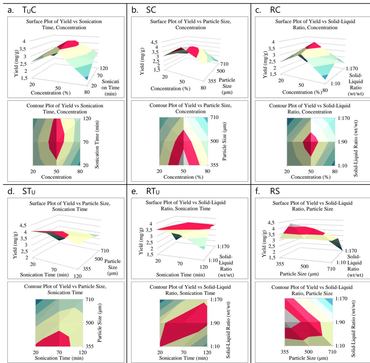
**Figure 4:** The surface and contour plots for rutin yield with UAE using male papaya leaves under the influence of (a) sonication time and ethanol mixture concentration, (b) size of plant matrix and ethanol mixture concentration, (c) solid-liquid ratio and ethanol mixture concentration, (d) particle size and sonication time, (e) solid-liquid ratio and sonication time, and solid-liquid ratio and (f) size of plant matrix.
