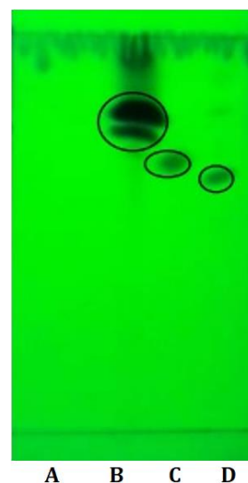
Figure 2: Confirmation of MH2011 purity using thin-layer chromatography. Silica gel GF254 was used as a stationary phase and chloroform:methanol (3:1) were used as a mobile phase. From left to right are urea (A), 4-amino-1-naphthol, RF 0.16 and 0.22 (B), p-aminophenol; RF 0.27 (C), and MH2011; RF 0.33 (D), respectively.
