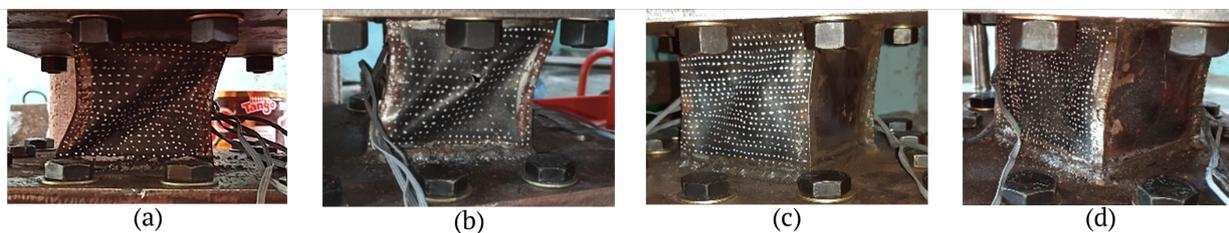
Figure 6 The deformed shape of the S-58.8 specimens in buckling state under load angles: a) 0°, b) 15°, c) 30°, and d) 45°.
