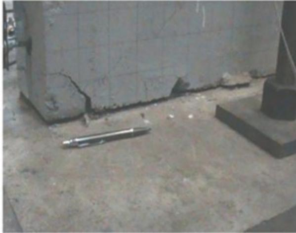
(a) Tie beam and foundation separation of experimental specimen (Triwiyono et al., 2020)
