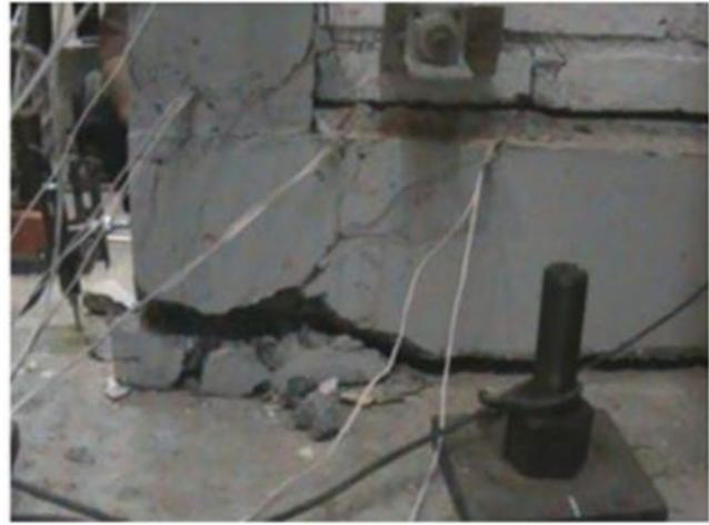
(b) Spalling at the bottom corner of the concrete frame (Triwiyono et al., 2020)
