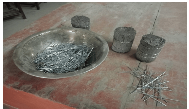
Figure 2. Steel fiber used in this investigation.
