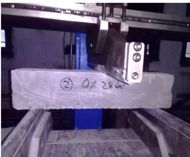
Figure 4. Flexural strength apparatus.
