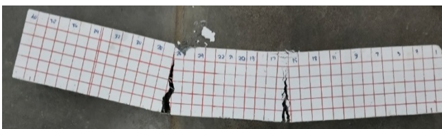
Figure 6 Crack pattern at ultimate failure load ( P_{ult} ) for beam with 5 \text{ kg/m}^3 PP fibers (PP5), exhibiting widely distributed narrow cracks consistent with highest ductility index.
