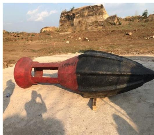
Figure 1. The DDC Hammer (9.7-ton weight)
