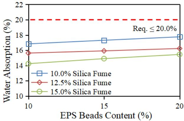
Figure 4. Water absorption of specimen
