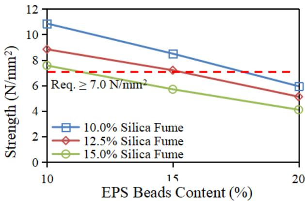
Figure 2. Compressive strength of specimens
