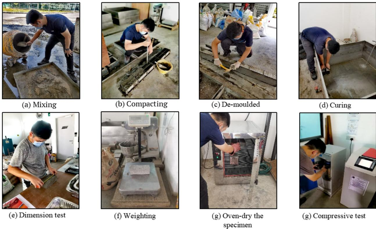
Figure 1. Preparation and testing
