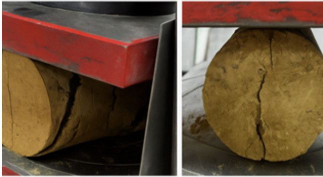
Figure 7 Indirect tension test
