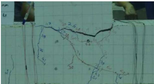
Figure 7. Crack Pattern of the Compressive Load (-), 24 mm
