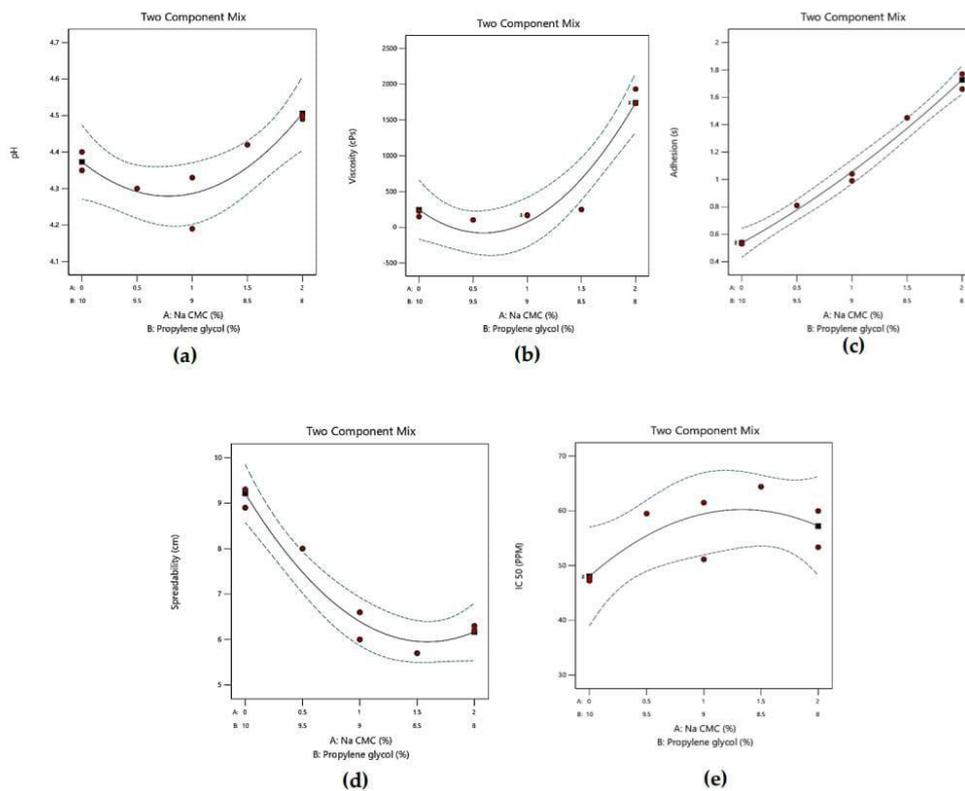
**Figure 2.** Graph of Effect Different Concentrations of Na CMC and Propylene glycol on Characteristic Test and Antioxidant Activity of Chicken Bone Collagen Antioxidant Gel Serum Based on Simplex Lattice Design : (a) pH (b) Viscosity (c) Adhesion (d) Spreadability (e) IC<sub>50</sub>
