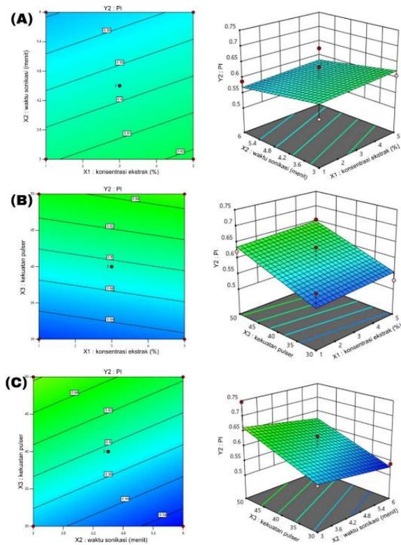
**Figure 3.** Response graph of the relationship between the independent variable (X) and the polydispersity index result (Y<sub>2</sub>)
