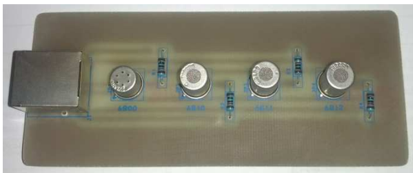
Gbr. 4 Array Sensor TGS
