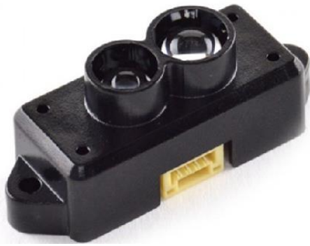
Fig. 1 Example of a LiDAR sensor.
